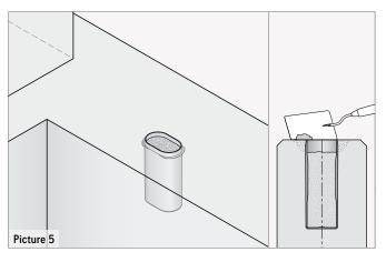
Prior installation the Concrete pocket in the lower unit must be filled with grouting mortar (picture 5), so that the steel bolt will set into the mortar during lowering of the upper unit (picture 6).
