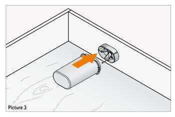
The corresponding holders for the Rebar and Concrete pocket are fixed to the mould by nailing, screwing or hot bonding. Afterwards the pockets are clipped on their fixed holders (picture 3). Those holders can be removed during demoulding easily.
