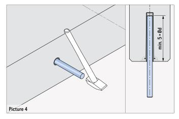
Before installation of the concrete elements, the steel bolt shall be firmly inserted into the Rebar pocket (min.  $5 \times \emptyset d$ ), in order to prevent it from falling out when mounting. The length of the steel bolts is to be calculated according to the installation situation.
