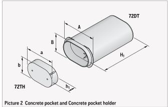
The Dowelling system is used for the fixation of two concrete units which are stacked. It consists of a rebar pocket - available in three sizes - for the upper concrete unit, a Concrete pocket for the lower concrete unit and a bolt made of reinforcing steel or
