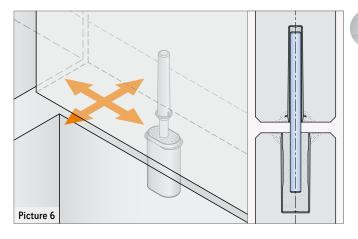
Because of the shape and size of the oval Concrete pocket, the elements can be aligned easily and sufficiently.
